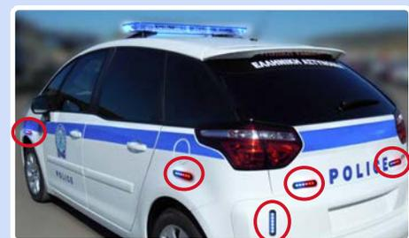
The NanoLED emergency warning light increase security due to both its reduced dimensions, and its several and simultaneous mounting positions, which magnify the vehicle's visibility.
